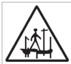
Danger Scaffolding Incomplete
