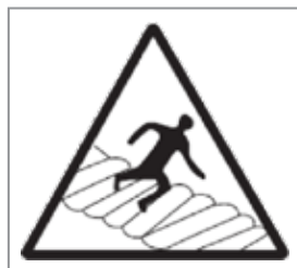
Danger Fragile Roof
